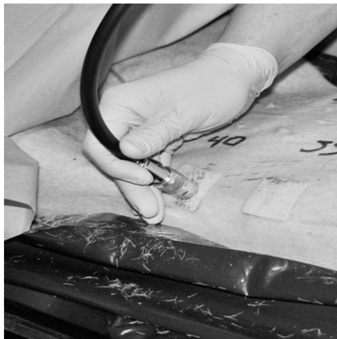
Figure 5. Performance of a dielectric measurement with a 5 mm probe.
